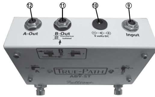
**Input:** (see #9 on above diagrams) Connect a cable (shielded with 1/4" mono plugs) coming from your guitar, bass, or other instrument into this jack. Always use good quality *shielded* cables (eg. Fulltone Gold Standards) for audio signals, speaker cables are *un-shielded* and should not ever be used to connect your instrument.
